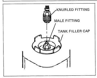
3. Connect fuel supply hose to gas tank outlet fitting. Pull back on the knurled sleeve, insert hose fitting over tank outlet fitting and let the sleeve snap into place to lock.
